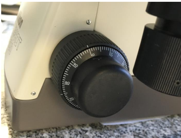
Focus knob with scale
